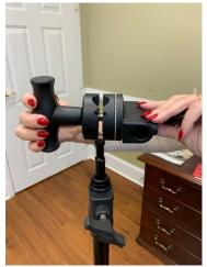
\*LOOSEN KNOB MIDDLE WAY DOWN EXTENDER POLE. SLIDE INTO LOWER POLE. LOOSEN KNOB AT BOTTOM OF POLE AND REMOVE EXTENDER POLE. PLACE IN CASE AND PLACE FOAM 3 OVER END OF POLE.
